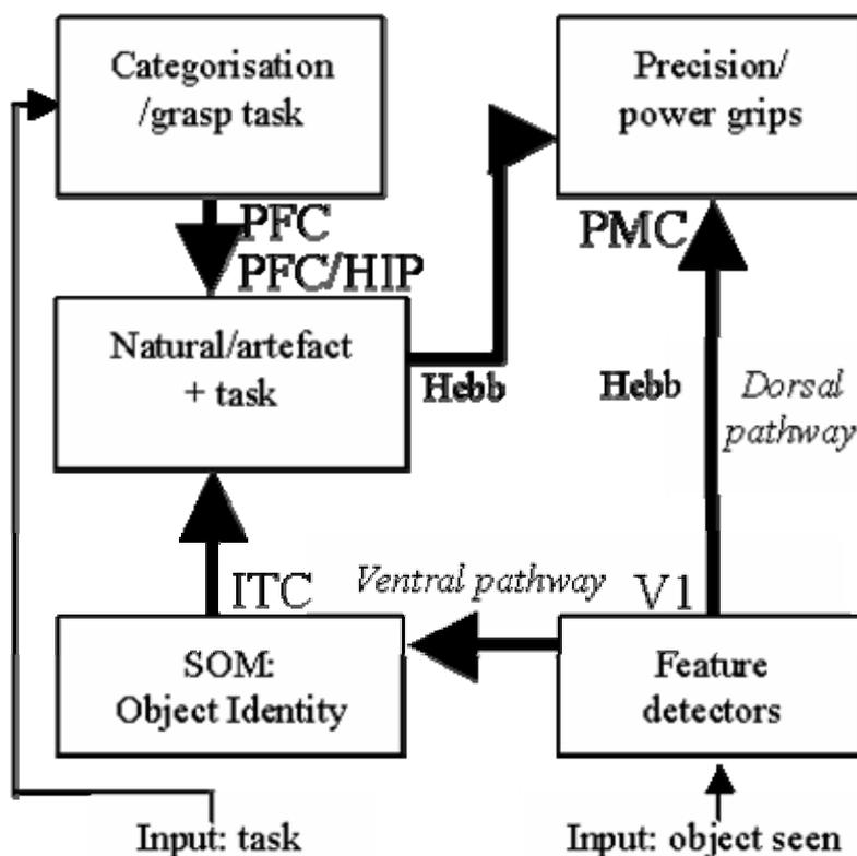
**Figure 1.** The architecture of the neural controller.
